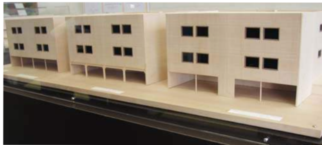
Models of Woodframe Apartment Buildings with Tuck-under Parking. [SHOWN LEFT]: no added seismic bracing; [CENTER]: steel moment-resisting frames added; [SHOWN RIGHT]: shear wall added
